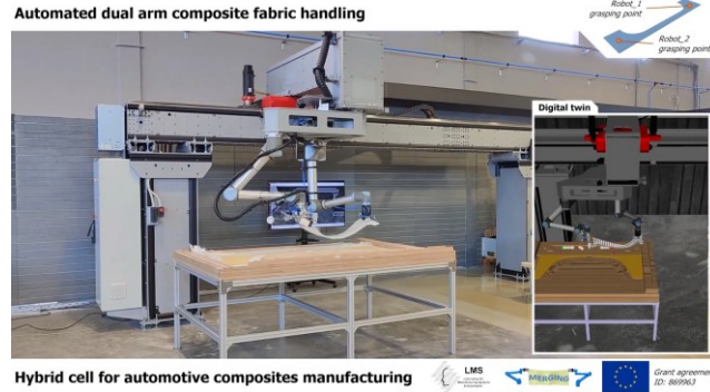
Automated dual arm composite fabric handling
