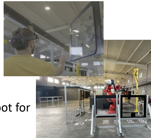
Digital Twin and AR-based tools for intuitive HRI - Bus windows assembly
