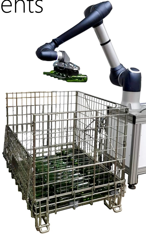
Collaborative boxing and deboxing robot for winery
